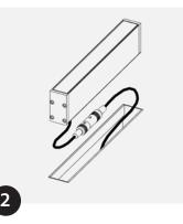
Make power connection to suit IP requirements of installation location. Insert MOMO-F.
